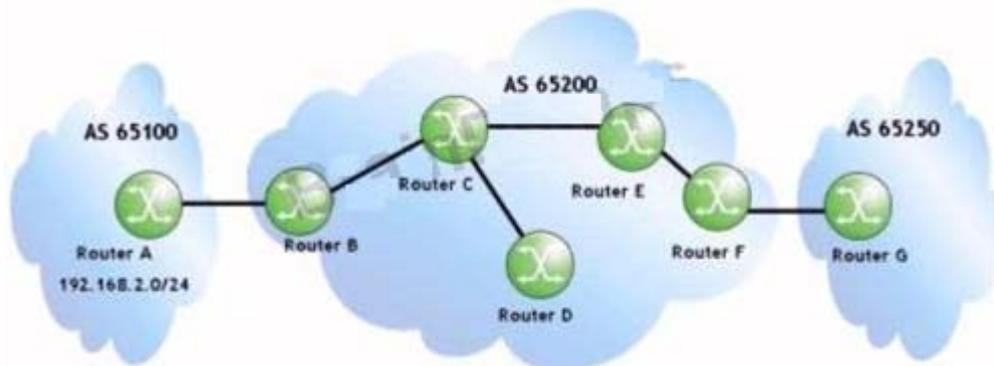
True or False: If router C and router E are route reflectors, and the lines in the diagram represent BGP sessions, this is a valid configuration.
