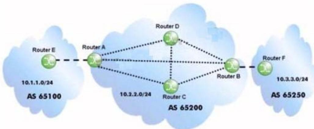
After router A receives the BGP update for the 10.3.3.0/24 prefix, which routers will the route be propagated to?
